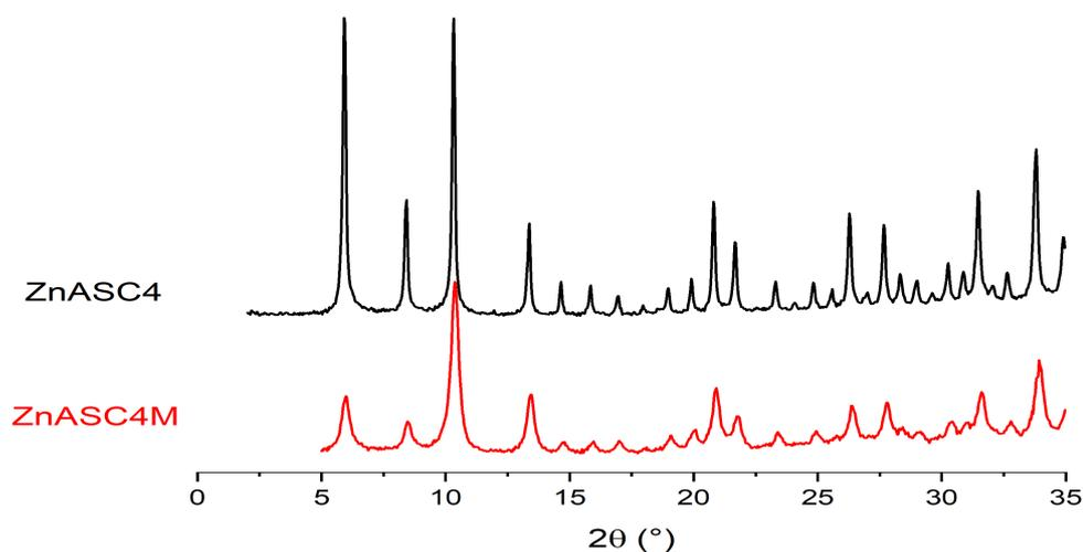
Figure 1. Comparison of X-ray diffraction patterns of ZnASC4 as synthesised, activated and ZnASC4M.
