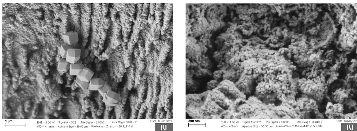
Figure 2. SEM photo of ZnASC4 crystals. Figure 3. Nano-MOF crystals of ZnASC-4M sample.
