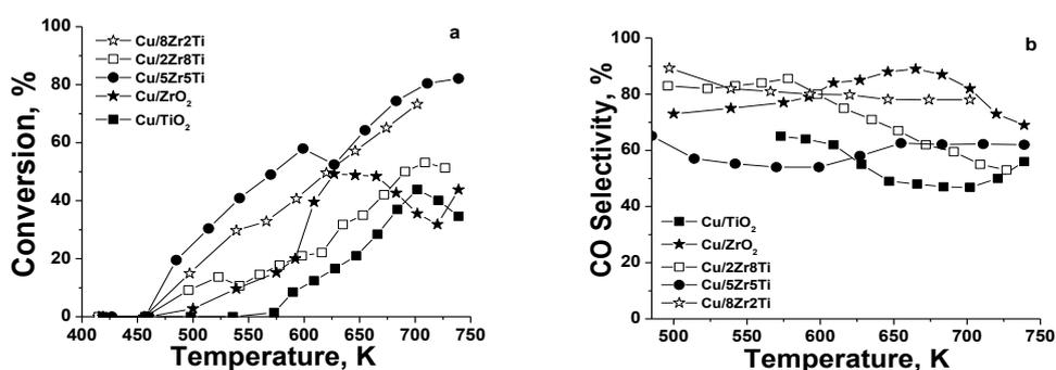
Figure 2. Methanol conversion (a) and selectivity to CO (b) of Cu/Zr-Ti materials
