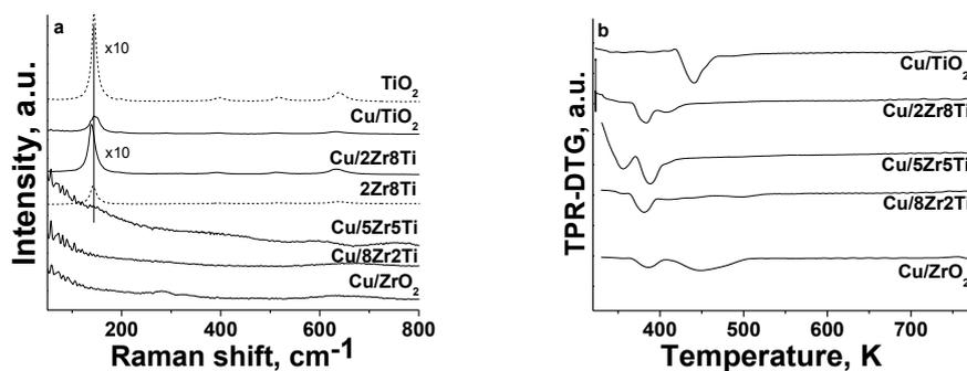
Figure. 1 Raman spectra (a) and TPR-DTG (b) of Cu/ZrTi materials.
